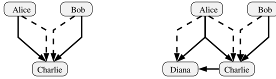
Fig. 2. Static trust graph for the example application. Solid edges denote confidentiality, while dashed edges denote integrity. The left graph depicts the initial static situation, the right hand graph the situation after Diana has joined the network.
